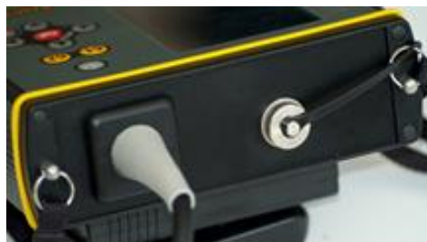
Photo 1a. Probe cable socket. PC transmission port
